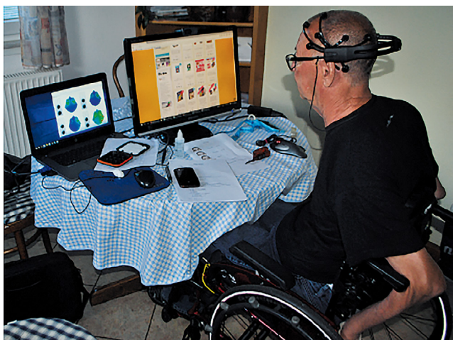
Fig. 5. Computer control by head movement [22]
